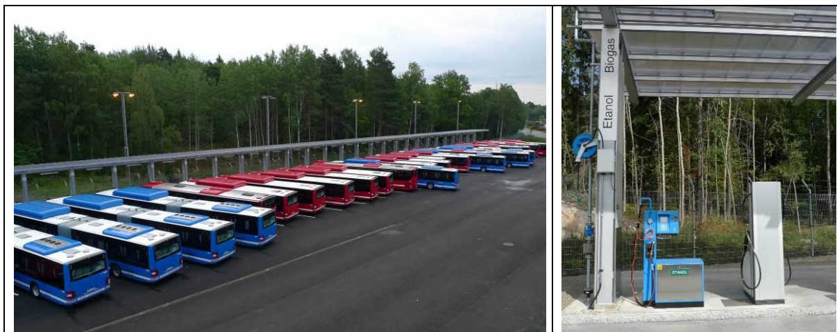
Figure 6. Left: Buses on slow filling ramp. Right: Dispenser for fast filling at Gubbängen, Stockholm.
